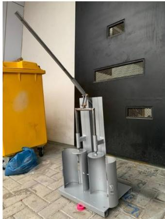
Gambar 11. Alat Press *Baglog*
