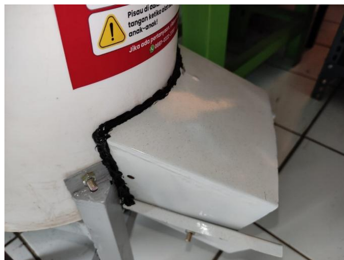
Fig. 7 Application of sealant on the joint gap between the shredding drum and outlet chute
